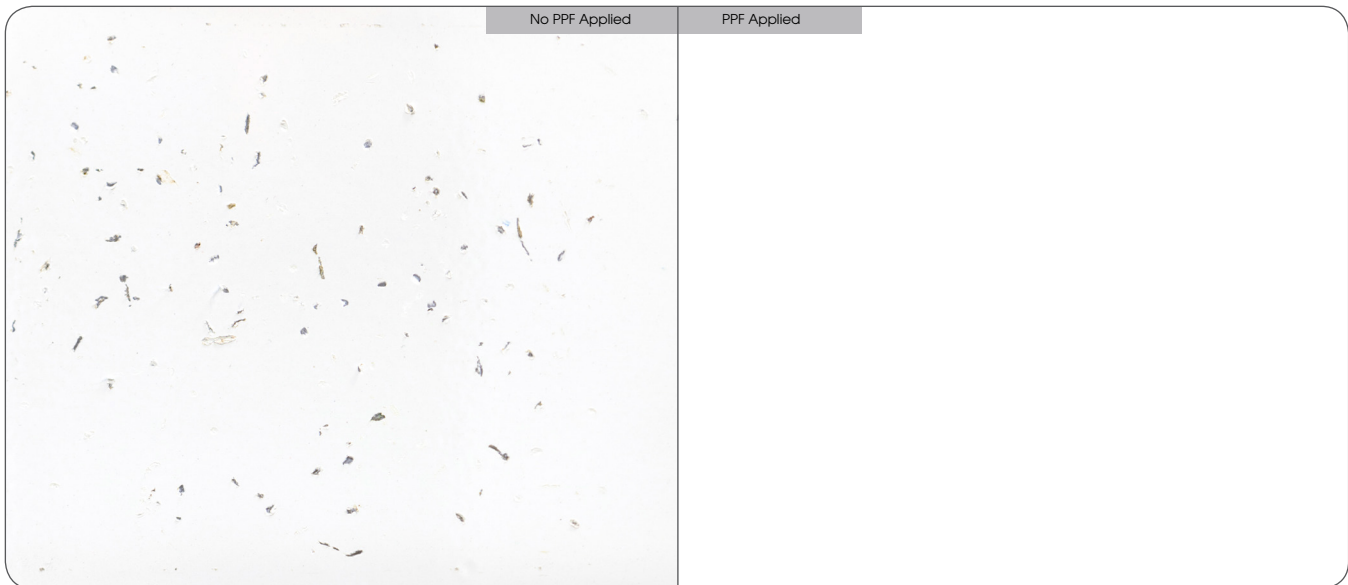
* Image represents gravel impact testing on surface with and without PPF installed
