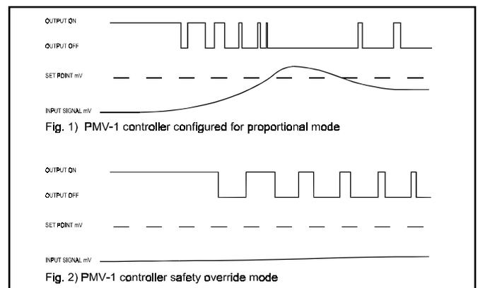
Low and high setpoints can be selected for the alarm relay. This relay may also be used as an additional set point.
