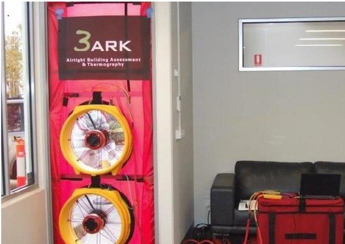
*This image shows our equipment as set up for a live assessment of the air tightness in a commercial building.*
