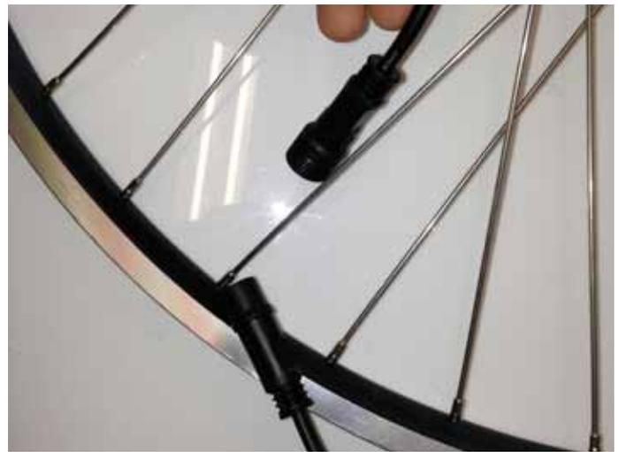
Find the connector on the motor lead and disconnect. This will allow you to attach the wheel to your bike with ease.
