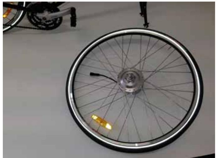
Remove the original front wheel from your bicycle and swap the tyre and tube from your old wheel to your new wheel. We recommend a thorn proof tyre and tube.
