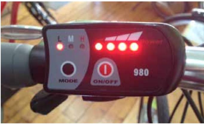
To turn your electric system on, start by making sure the battery is switched on. This can be seen on the previous page. Once Battery is on press the On/Off button on the display. The Mode button changes the pedal assist level. The four red LED's lit up in the photo are the battery level indicators.
