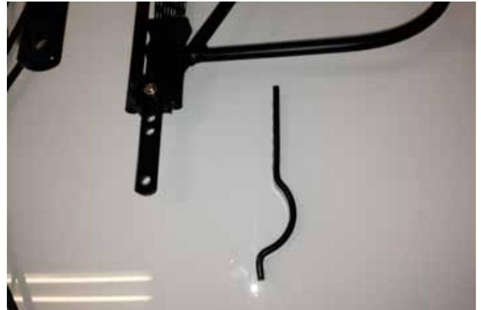
To attach the battery rack your bike must have rack mounts. Most bicycles have these mounts. The Power-Ped battery rack comes with multiple adjustments. You will find a spare rack leg (as seen above). Attach this leg to the rack if you have a disc brake on the rear. You can also adjust the arms so the rack fits to your bike neatly.
