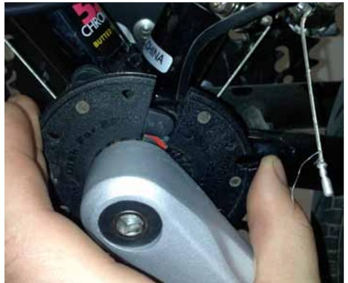
Next you will need to attach the magnet wheel to the bottom bracket axel on the left hand side as shown above. Once clipped in, place the outer ring on the outside of the magnet wheel to secure.
