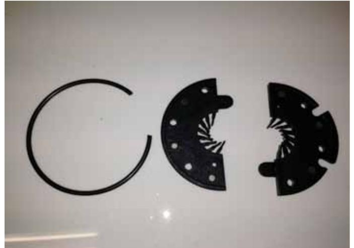
The pedal assist system allows you to power your motor using pedal power. It's controlled by the pedal assist display on the handle bars. On the display you can turn the pedal assist on/off and choose from 3 different speed options. To attach the sensor and magnet wheel start by separating the 2 halves of the magnet wheel.
