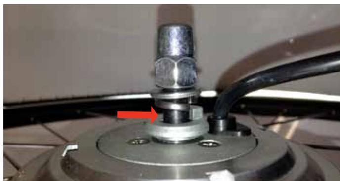
The red arrows above show you where the fork drop out should be attached. Make sure the hook on the hook washer is sitting at the bottom of fork dropout. In some cases the fork drop out might need to be lightly filed in order for the motor axel to fit. If you are having trouble fitting the axel in the fork drop outs you can use a 10mm spanner to manipulate the axle. You can also take off the outer nuts and washers to make attachment easier.
