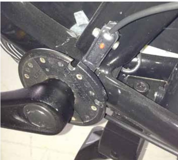
To attach the sensor you will need to first line it up with the magnets on the wheel. Once you have found the appropriate position for the sensor, peel the adhesive plastic off the back and attach sensor to frame. It is best add some zip ties to fully secure the sensor.
