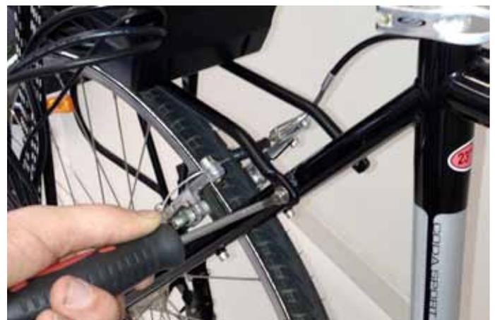
Find these rack bolts in the packaging, Attach the rack by putting it in place and screwing the screws into the rack mounts. For extra strength and tightness use lock tight.
