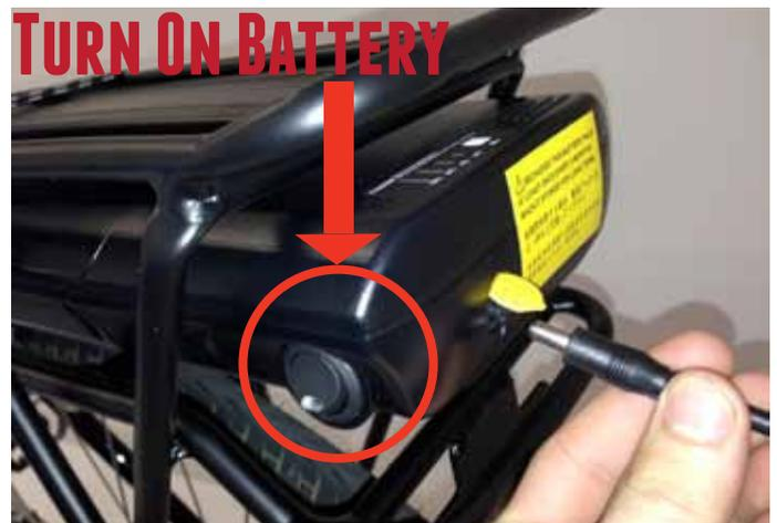
To charge the battery, remove the charger from it's packaging and plug the power cable into the wall and the charger. Take to phono connector and plug it into the charging port found on the rear of the battery under the yellow flap.
