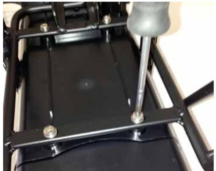
It's a good idea to double check the tightness of the bolts that hold the plastic battery casing to the rack itself. These bolts can come loose in rough terrain so make sure they are done up reasonably tight.
