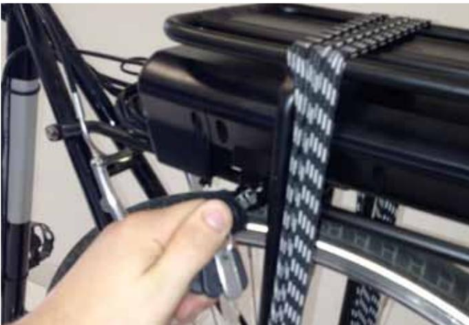
To unlock battery and remove from bike, rotate the key clockwise. The lock can be found on the left hand side of the battery rack. Once rotated, you can slide the battery out of the rear of the rack. Be sure to double check the battery is locked before riding to avoid an expensive mistake!
