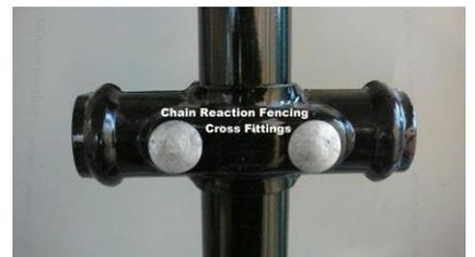
**Top, Middle and/or Bottom rails with cross fittings (optional)** - Measure the inside distances between each set of posts and deduct 30mm to allow for the fitting bolts. Mark the measurement on the rail and cut with a metal cutting tool as required. Bolt rails on using cross fittings (see image above right).
