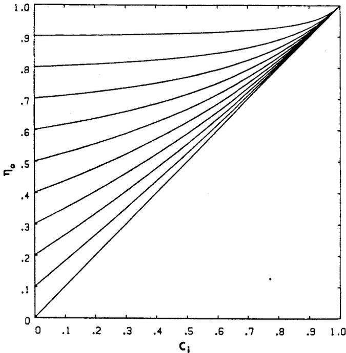
Fig. 4.—Effect of cross by-pass flow into inlet,  $C_i$ , on the overall effectivity of a regenerator side,  $\eta_o$ , for a range of values of regenerator effectivity,  $\eta_r$ , given by  $\eta_o = \eta_r$  at  $C_i = 0$ .
