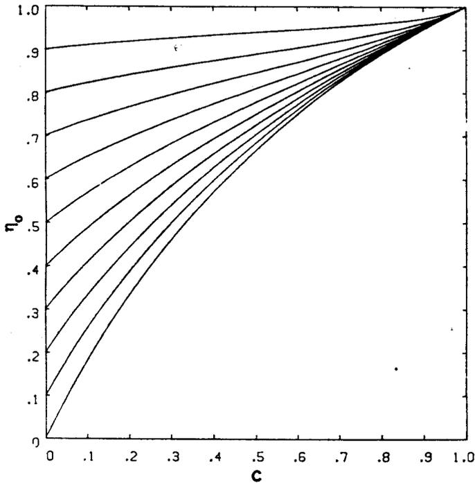
Fig. 7.—Effect of equal cross by-pass flows into inlet and outlet,  $C_i = C_o = C$ .
