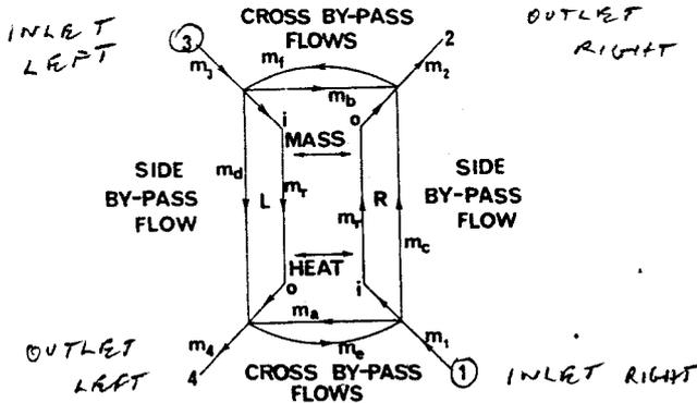
Fig. 3.—Transfer and mixing model of a regenerator with by-pass flows.
