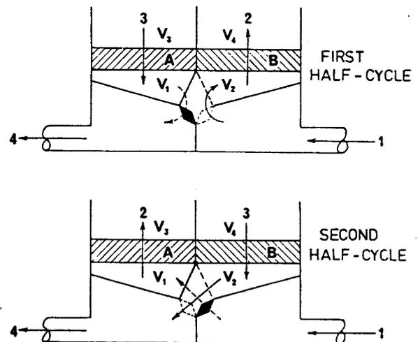
Fig. 2.—Switched-bed regenerator. Full and broken lines show sections through the different halves of the regenerator length.
