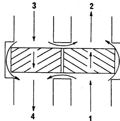
Fig. 1.—Rotary regenerator with by-pass flows.
