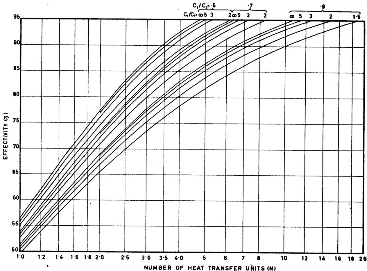
Fig. 3.—Heat Transfer Effectivity  $\eta$  for Flow Stream Capacity Rate Ratio  $C_1/C_2 = 0.9, 0.7$  and  $0.5$ , and  $h_1 A_1/h_2 A_2 = 1$ .
