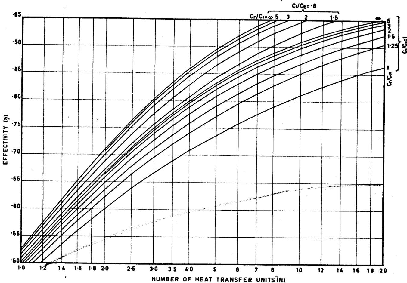
Fig. 2.—Heat Transfer Effectivity  $\eta$  for Flow Stream Capacity Rate Ratio  $C_1/C_2 = 1.0$  and  $0.8$ , and  $h_1 A_1/h_2 A_2 = 1$ .
