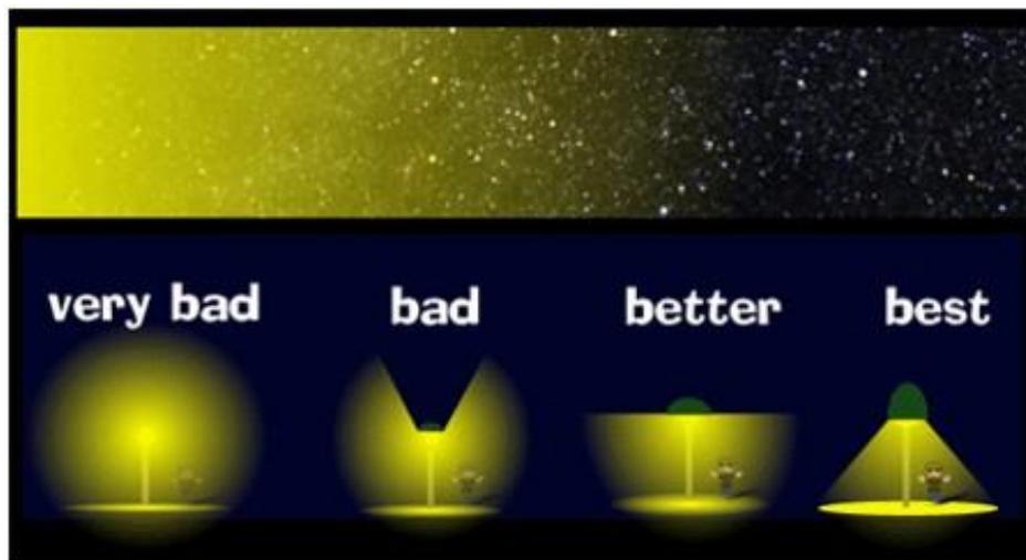
Good lighting shines down where it is needed for security, not up into the sky where it is wasted and prevents star gazing
