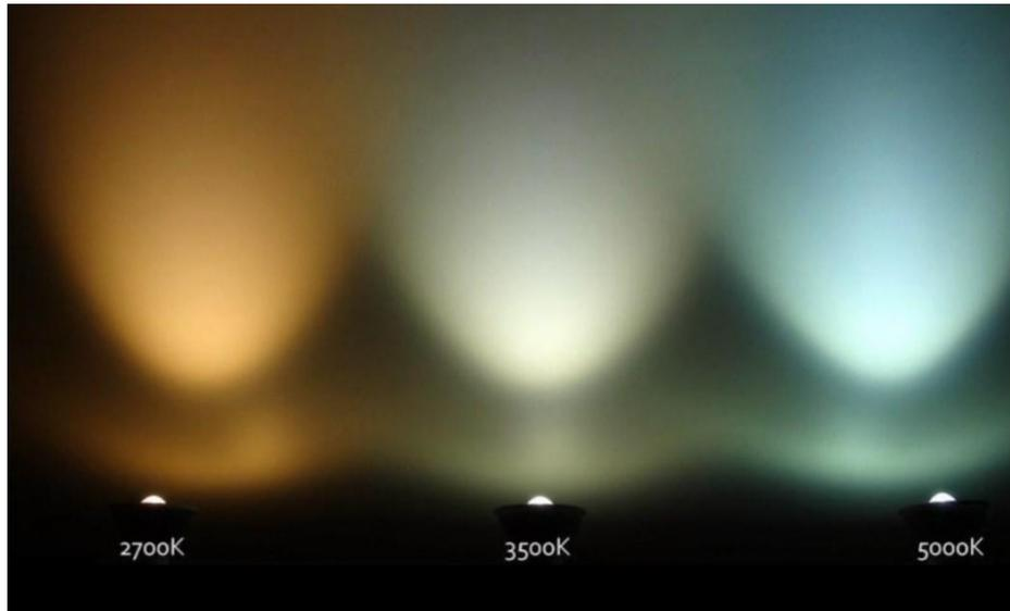
Good lighting uses lamps with a warm yellow or orange colour, as specified by a low colour temperature
