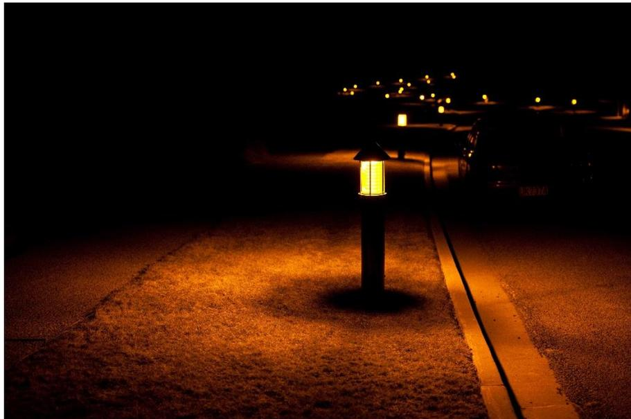
Light bollards such as this one at Lake Tekapo are ideal for a Dark Sky Park or Reserve. Note that the light shines on the ground where it is needed and not directly into our eyes. The light colour is yellow or orange, which has less impact on human health, on the environment and on our ability to see the stars.
